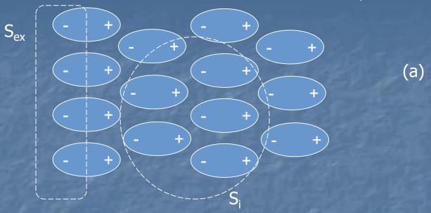
Within the dialectic, over macroscopic volumes  $(S_i)$ , the net charge is zero, while on the surface of this volume  $(S_{ex})$  a net charge is accumulated (induced) and causes the electric dipole of the entire substance.
