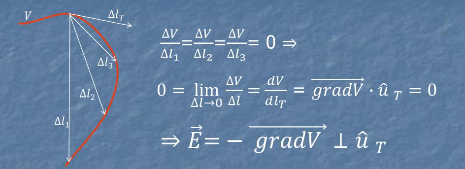
The electric field lines (flux) is always perpendicular to an equipotential surface and hence work done in moving a charge between two points on an equipotential surface is zero.
