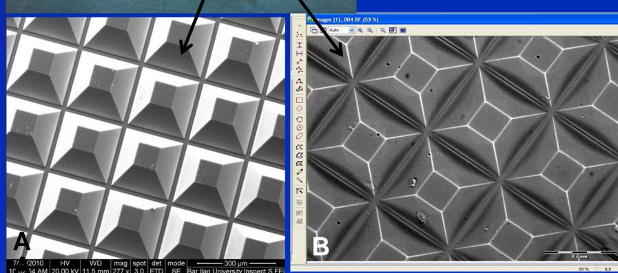
**SEM image of the PDMS master (A) used for MCs embossing in agarose. Each MC (B) is designed to accommodate a single 3D spheroid (magnification ×10). MCs' pitch is 250 μm and depth is about 100 μm.**
