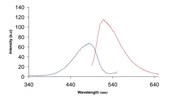
Figure 3. exitation (blue) and emission (red) spectrum of 10uM BO21 in water.
