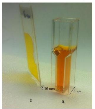
Figure 2. 8mM dye concentration in the two cuvettes, a) 10 mm width cuvette. b) 0.15mm width cuvette.
